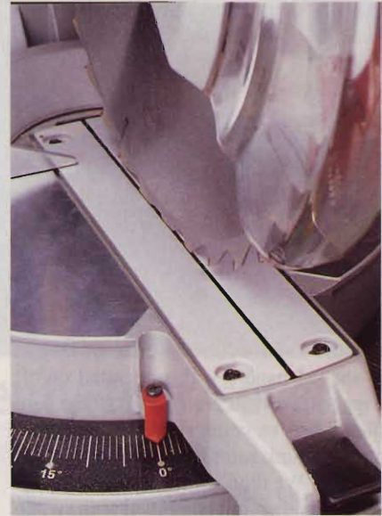
Right: Makita's two-piece insert allows you to narrow the blade opening to reduce tearout or open it for bevel cuts.
